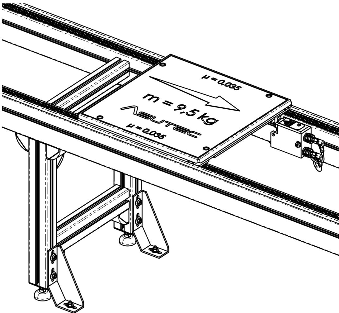
Calculation:  $F_{R\min} = m_{\min} \cdot g \cdot \mu_{\text{norm}} = 3\text{kg} \cdot 9,81\text{m/s}^2 \cdot 0,07$   $F_{R\min} = 2,06\text{N}$
